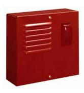
**S/EKO F24:** Self powered outdoor sounder with flash, IP34, 24Vdc. Multi-tone piezoelectric sounder with high acoustic power and high-visibility Xeno flashlight. Its classic and functional aesthetics is suitable for residential, commercial and industrial environments. Available in red for fire systems.
